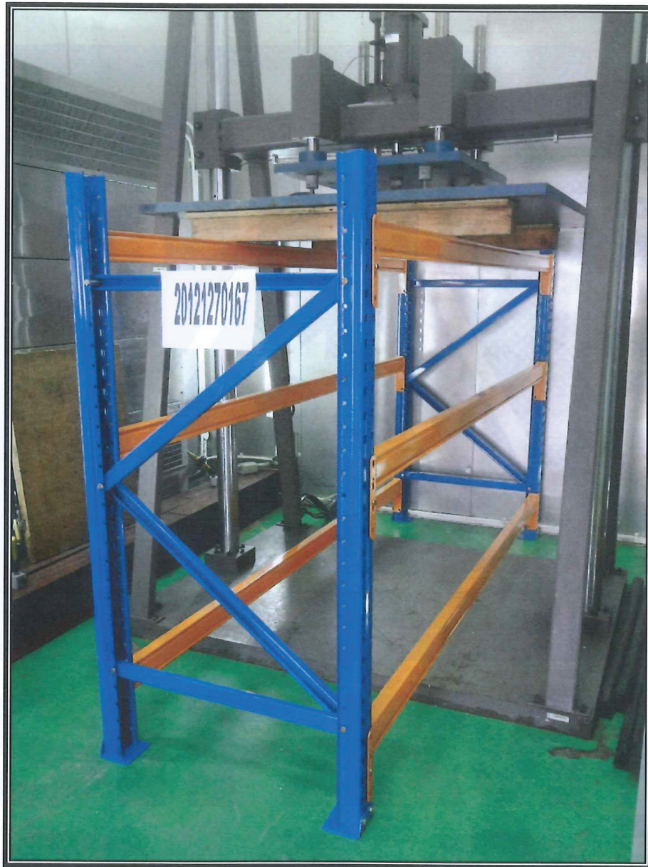
Compression Test Setup for Heavy Duty Pallet Racking
