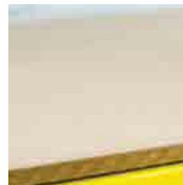
HDF BOARD : 8mm thick High Density Fiber
